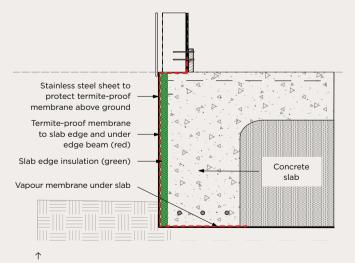
Construction detail for the installation of a membrane with integrated termiticide over slab edge insulation.
