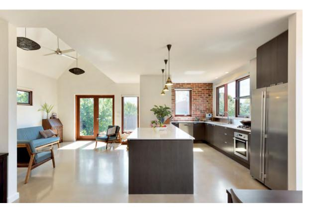
Sixty per cent of the cement component in the low embodied energy concrete slab is replaced with waste products slag and flyash. Windows in the northern and southern walls are aligned to channel summer breezes through living spaces for natural cooling and effective night purging. Eaves on the northern side are designed to provide solar access to the slab in winter and exclude the sun in summer. A profile of this Positive Footprints design is in Sanctuary issue 18. Image: Emma Cross
