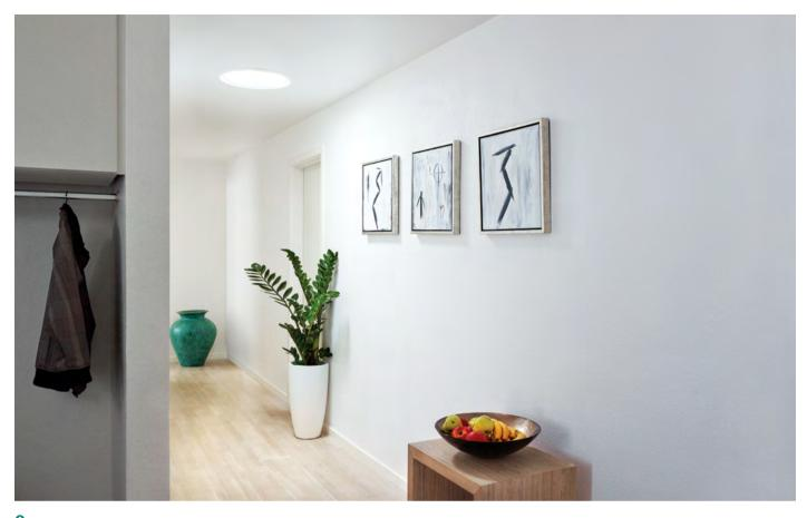
The advantages of tubular skylights are twofold: they can be located in slightly awkward and tight spaces where a conventional roof window or its shaft could never fit; and they cause very little heat gain or heat loss. Image: Velux
