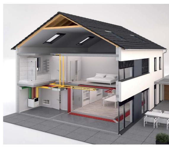
The yellow ducting shows where the moist, stale air is being extracted from wet areas; the red ducting illustrates the fresh, filtered air being delivered to bedroom and living areas. The heat exchanger uses the energy from the exhaust air (brown) to heat or cool the incoming outside air (green).
